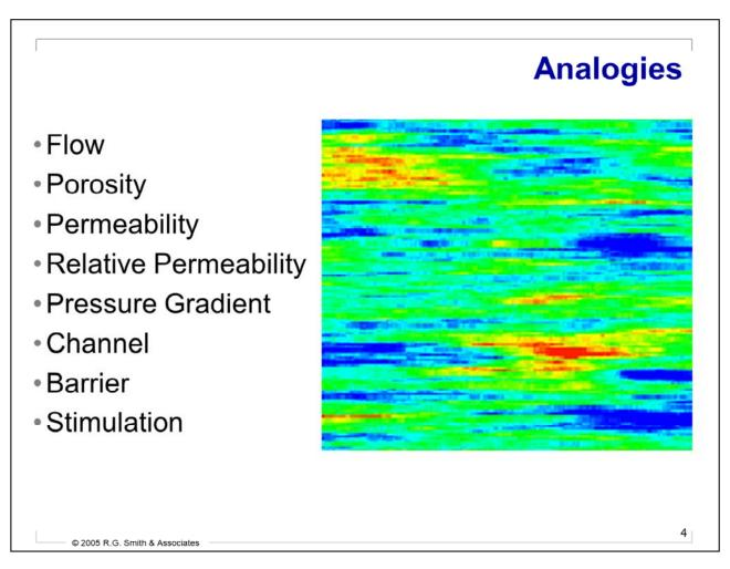
Two-dimensional slice through a petroleum reservoir (depth increasing from top to bottom). Red - Low Permeability; Blue - High Permeability.
